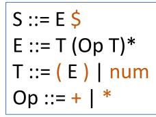
AST Construction Let's construct the syntax tree for 2 + (3 \* 4) \$ Apply: E ::= T Op T, Left: E=2, Op=+, Right: T=(3 \* 4)
